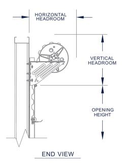
Universal mount 2.25" deep 16-gauge galvanized steel guides require no pre-installation modifications for wood, steel, concrete or filled masonry block
