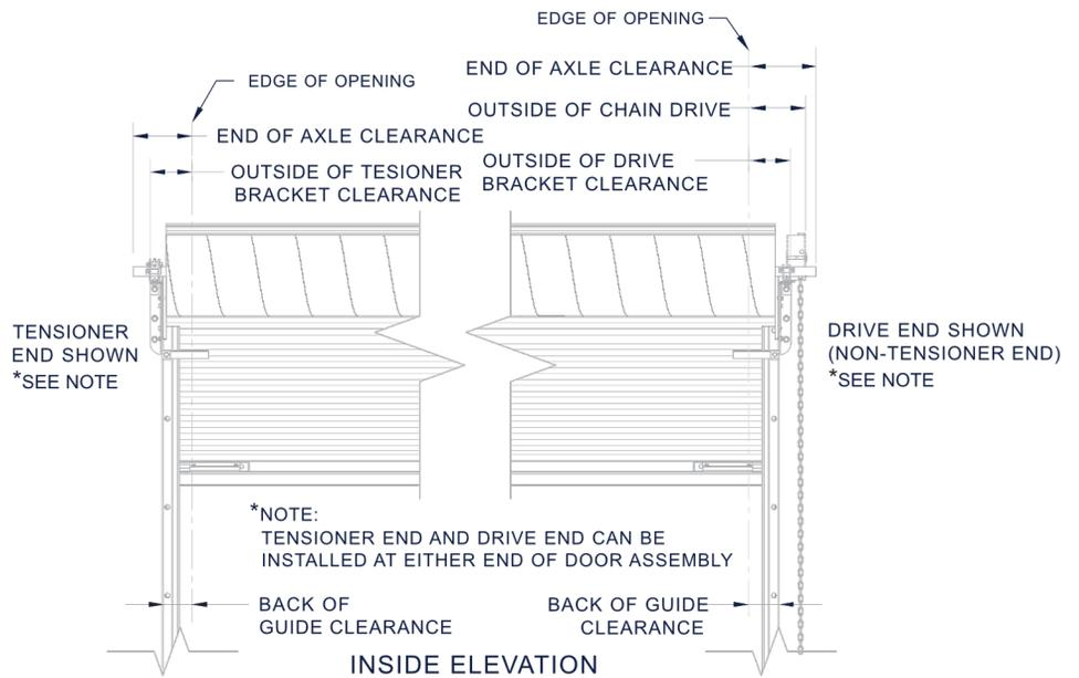
Universal mount 4" deep 12-gauge galvanized steel wind bar guides require no pre-installation modifications for steel, concrete or filled masonry block applications.
