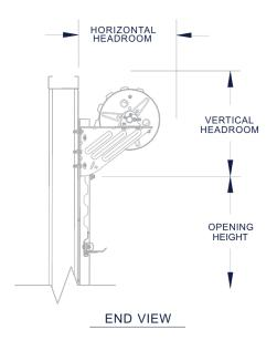
Universal mount 2.25" deep 14-gauge galvanized steel wind bar guides require no pre-installation modifications for steel, concrete or filled masonry block applications.
